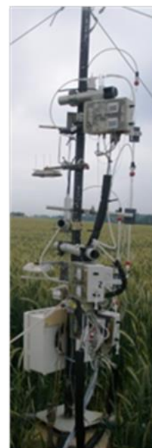
Figure M28.1. Left: Measuring the gradients of NO, NO 2 and O 3 at three heights using a continuous sampling pump, a multiplexer and gas analyzers (Stella et al. , 2012).
