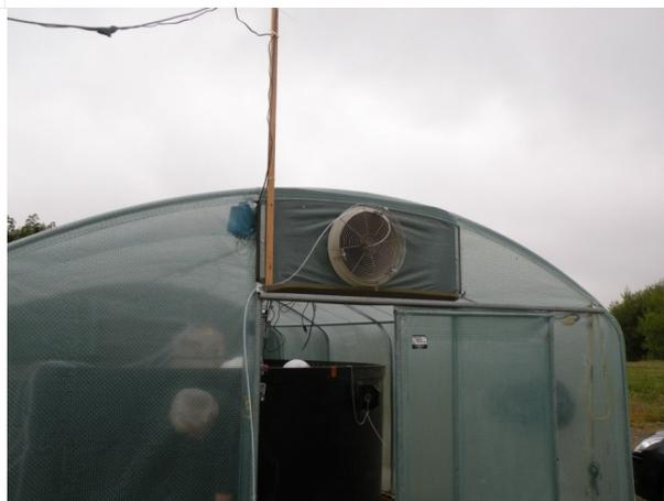
**Figure 20. The tank cover facilitated with: (1) Fancom fan with a calibrated 'Fancom Exavent®' ventilation rate sensor measured ventilation rates with an accuracy of 45m<sup>3</sup>/h. (2) array of temperature sensors to measure slurry temperature at different depths. (3) Temperature and humidity sensor to measure near surface air temperature and humidity**
