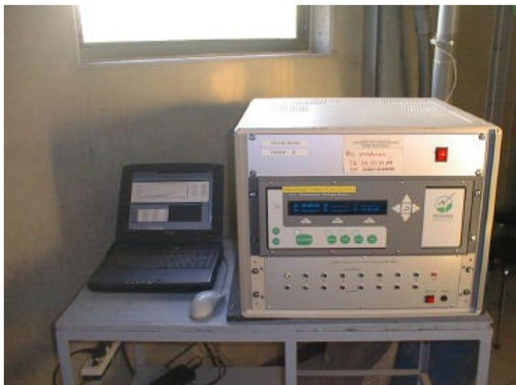
**Figure 39. Photo-acoustic multi-gas monitor with 6 channel multi-sampler**
